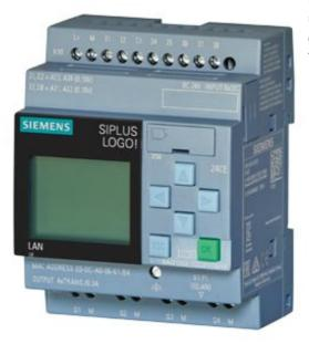
SIPLUS LOGO! 24CE -20...+70°C start up -20°C with conformal coating based on 6ED1052-1CC08-0BA0 . logic module, Display PS/I/O: 24 V/24 V trans., 8 DI (4AI)/4DO, memory 400 blocks, modular expandable, Ethernet integr. web server, data log, user-defined Web pages, standard microSD card for LOGO! Soft Comfort V8 or higher, older projects executable
