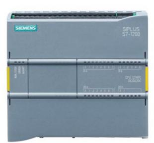
SIPLUS S7-1200 CPU 1214FC DC/DC/DC -25...+55°C with conformal coating based on 6ES7214-1AF40-0XB0 . compact "CPU, DC/DC/DC, ""onboard I/O: 14" "DI 24 V DC;"" ""10 DO 24 V DC; 2" "Al 0-10 V DC,"" Power supply: DC" 20.4-28.8 V DC Program/data memory 125 KB
