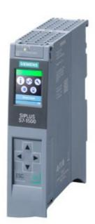
SIPLUS S7-1500 CPU 1511-1 PN -40°C+60°C with conformal coating based on 6ES7511-1AK02-0AB0 . Central processing unit with Work memory 150 KB for program and 1 MB for data, 1st interface: PROFINET IRT with 2-port switch, 60 ns bit performance, SIMATIC Memory Card required
