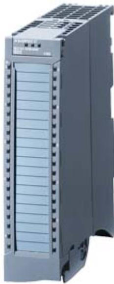
SIMATIC S7-1500 analog input module AI 8xU/I/RTD/TC ST, 16 bit resolution, accuracy 0.3%, 8 channels in groups of 8; 4 channels for RTD measurement, common mode voltage 10 V; Diagnostics; Hardware interrupts; Delivery including infeed element, shield bracket and shield terminal: Front connector (screw terminals or push-in) to be ordered separately
