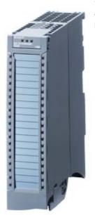
SIMATIC S7-1500 Analog output module AQ 4xU/I ST, 16 bit resolution, accuracy 0.3%. 4 channels in groups of 4; Diagnostics; Substitute value; Delivery including infeed element, shield bracket and shield terminal: Front connector (screw terminals or push-in) to be ordered separately
