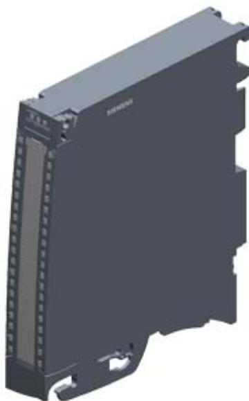
SIMATIC S7-1500 Analog input/output module AI 4x U/I/R/RTD/TC ST; 4 channels in groups of 4; Hardware interrupts; Diagnostics AQ 2x U/I ST; 2 channels in groups of 2; Substitute value; Diagnostics Common mode voltage approx. 10 V 16 bit; Accuracy 0.3%; Delivery including push-in front connector, infeed element, shield bracket and shield terminal
